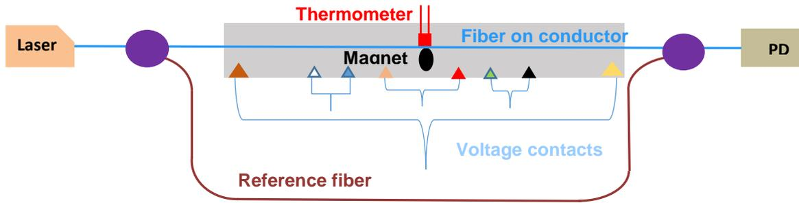
Figure 1. Experiment setup schematic
