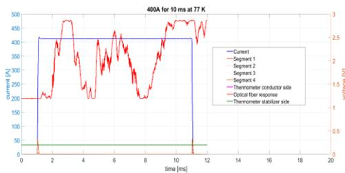
Figure 2. Experiment results showing optical fiber output for no quench
