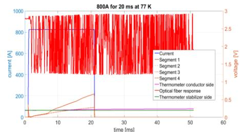
Figure 3. Experiment results showing oscillations in optical fiber output with quench
